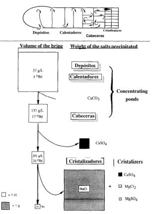
Figure 2. Graphic representation of the brine flow and the evaporation and precipitation processes in Spanish coastal salinas. The names of the different evaporation ponds are given in Spaniah and in English.
